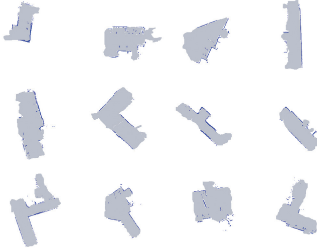
Fig. 6. Scan measurements, obtained by concatenating scans from around landmark locations, used by the RBPF algorithm.
