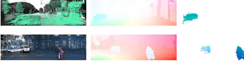
Fig. 4. A visualization of motion hypothesis (left), optical flow (middle), and scene motion flow (right). Camera motion is explicitly removed from scene motion flow. In the image of the cyclist we show that although multiple motion hypotheses are discovered by RANSAC (in two colors), a final smooth motion over this non-rigid entity is estimated with continuous optimization.
