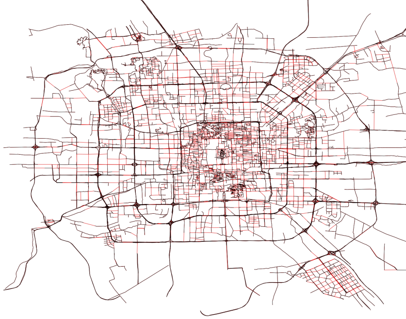
Figure 1: The main idea in this paper is to combine the advantages of direct and iterative methods: we identify a subgraph that can easily be solved using direct methods, and use that as a preconditioner in conjugate gradients. This is illustrated above with a map of Beijing, where the subgraph is a spanning tree (in black), and the remaining loop-closing constraints are shown in red.
