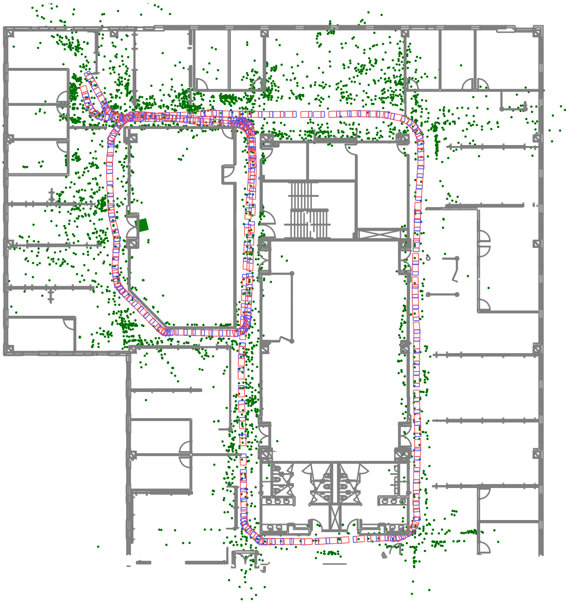
Figure 16: Projected trajectory and map after applying incremental \sqrt{\text{SAM}} using visual input and odometry only. Each robot pose is shown as an outline of the ATRV-Mini platform. The recovered 3D structure is represented by green points. For comparison the manually aligned building map is shown in gray. Given that no loop-closing occurred and considering the large scale of the environment and the incremental nature of the reconstruction method, this result is of very high-quality. Note that features also occur along the ceiling, and that some features outside the building outline are caused by reflections.
