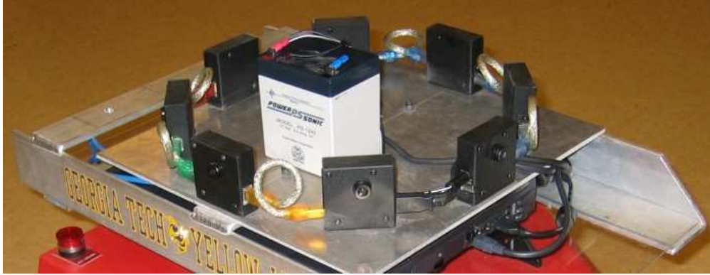
Figure 15: Custom made camera rig, mounted on top of an ATRV-Mini mobile robot. Eight Fire-Wire cameras are distributed equally along a circle and connected to an on-board laptop.
