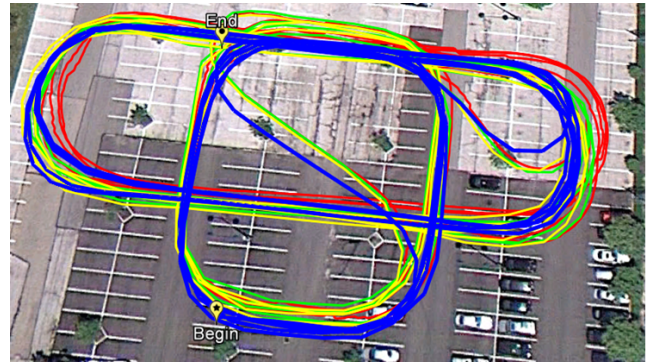
Fig. 6: Trajectories on parking lot scenario (1.74 kilometers): Ground Truth (blue), our short-term smoother solution (yellow, 3D RMS error: 2.11 meters), the first baseline method (red, 3D RMS error: 2.88 meters), and the second baseline method (green, 3D RMS error: 2.46 meters). Note the repeated loops stick tighter (such as the right portion of trajectories) in our solution.
