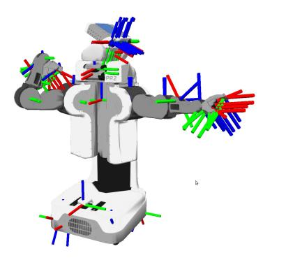
We rigidly attach coordinate frames to objects of interest. To specify the position and orientation of the object, we merely specify the position and orientation of the attached coordinate frame.
