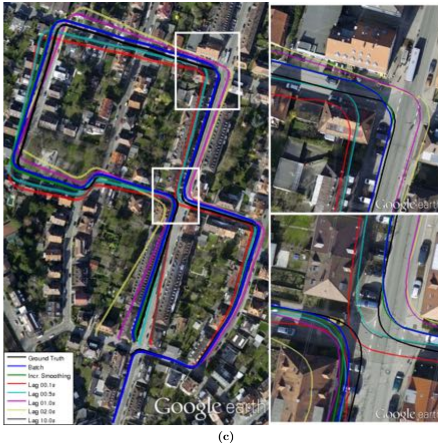
Figure 7.1: Aided inertial navigation [103]. (a) Factor graph for visual odometry integration with inertial bias estimation. (b) GPS integration (red factors) and/or stereo integration (blue). (c) Evaluation on KITTI sequence: Incremental smoothing performs almost as good as full batch optimization. Fixed-lag smoothing solutions are also shown for various lags.
