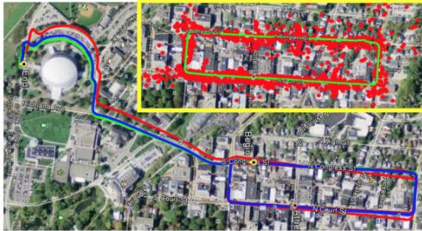
Figure 7.10: Large City Navigation Scenario (3.3 kilometers) from the DARPA ASPN project: Ground truth (blue), solution using only 1-step short-term smoother (red, 3D RMS error: 19.19 meters), solution using the CSM scheme (green, 3D RMS error: 5.85 meters), and the 3D landmarks constructed during the first loop (red points inside the highlighted yellow box).
