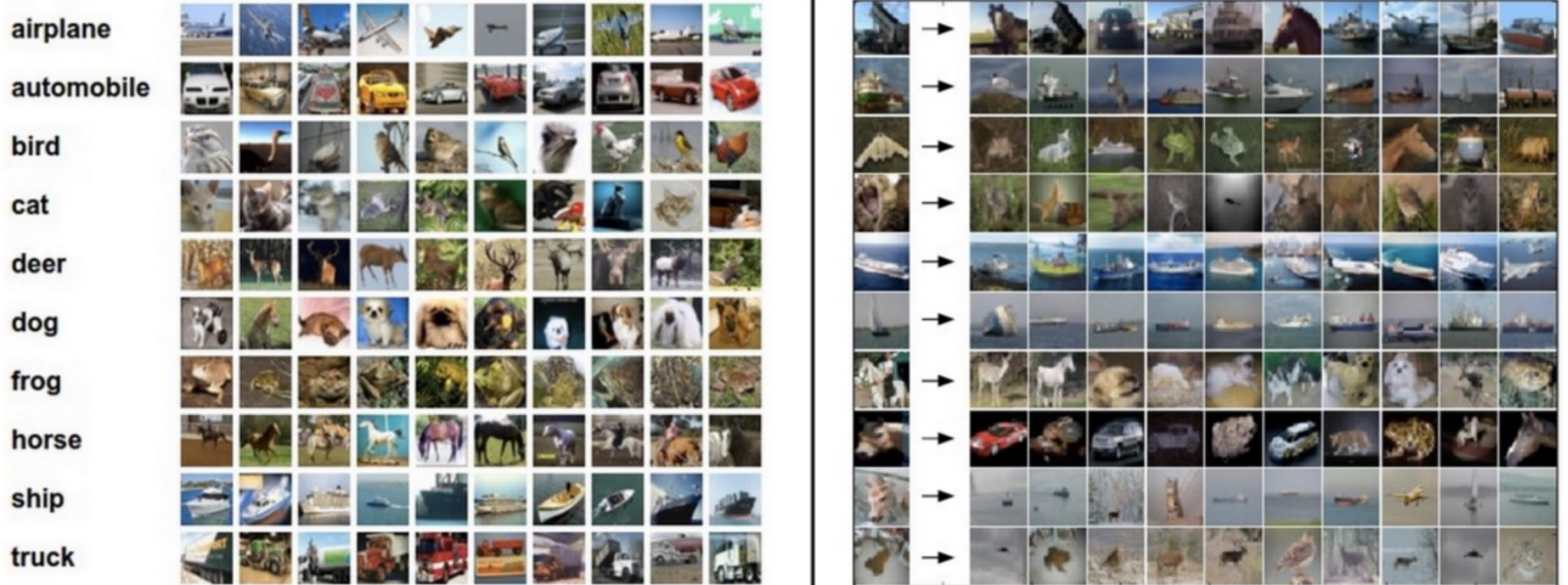
Left: Example images from the CIFAR-10 dataset . Right: first column shows a few test images and next to each we show the top 10 nearest neighbors in the training set according to pixel-wise difference.
