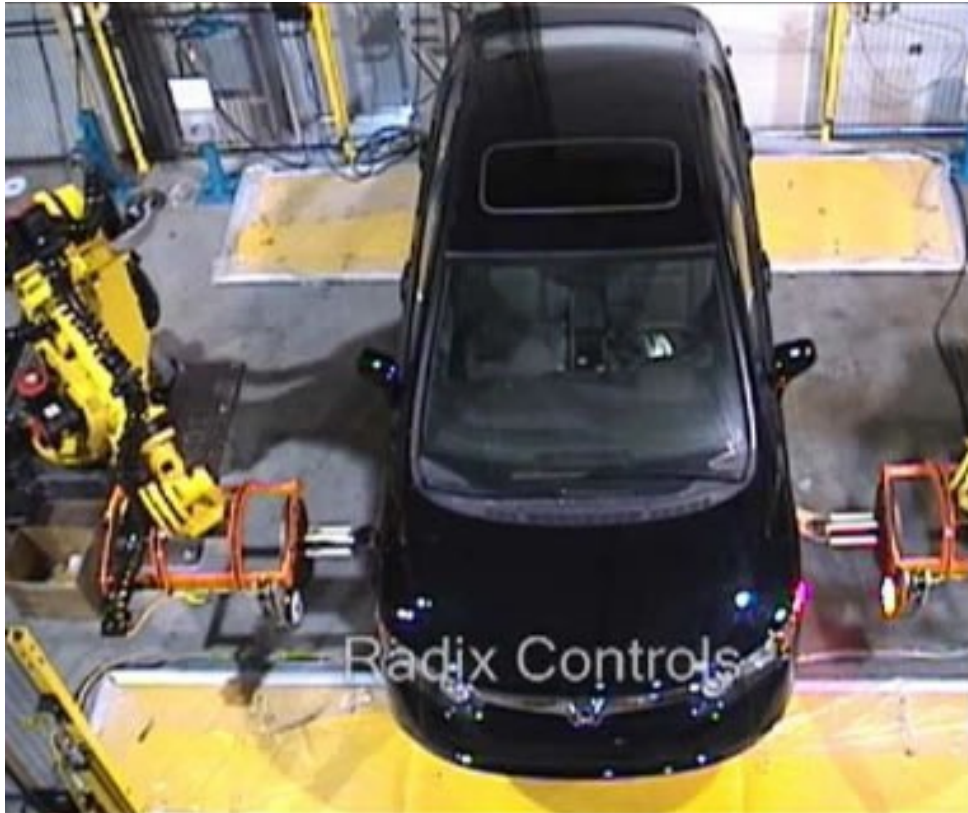
Vision-guided robots position nut runners on wheels
