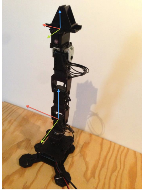
Figure 8.1: Pincher robot at rest, with all joint angles at 0. The chosen base frame S and tool frame T are shown as RGB coordinate frames.
