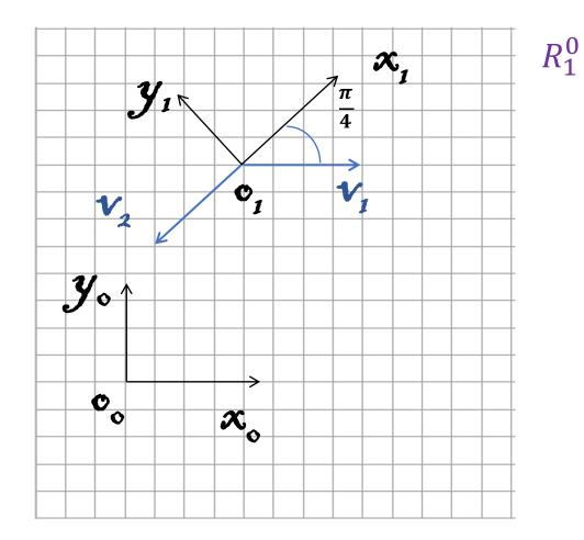
$$= \begin{bmatrix} 0.5\sqrt{2} & -0.5\sqrt{2} \\ 0.5\sqrt{2} & 0.5\sqrt{2} \end{bmatrix} \qquad R_0^1 = \begin{bmatrix} 0.5\sqrt{2} & 0.5\sqrt{2} \\ -0.5\sqrt{2} & 0.5\sqrt{2} \end{bmatrix}$$
