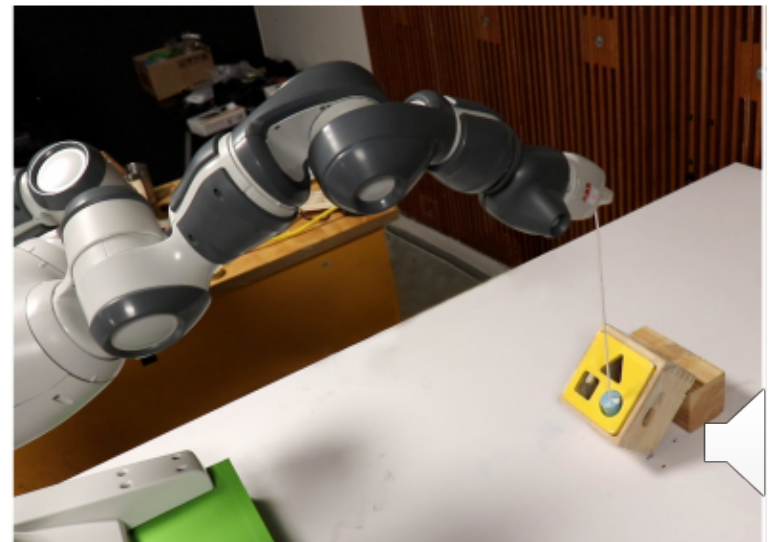
Fig. 1. Policies for opening a cabinet drawer and swing-peg-in-hole tasks trained by alternatively performing reinforcement learning with multiple agents in simulation and updating simulation parameter distribution using a few real world policy executions.
