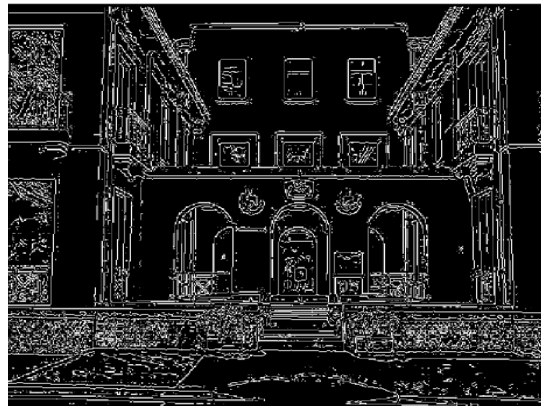
low threshold (weak edges)
