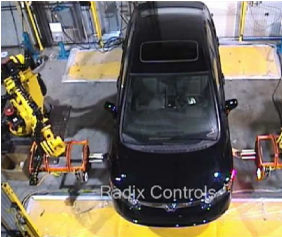
Vision-guided robots position nut runners on wheels
