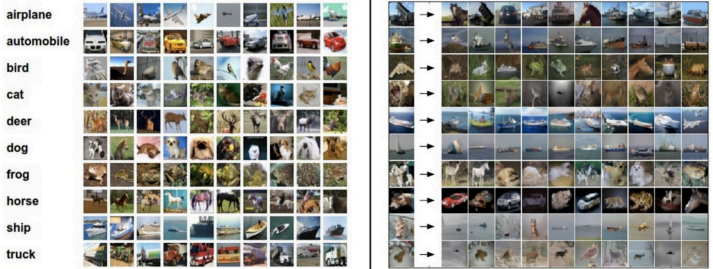
Left: Example images from the CIFAR-10 dataset . Right: first column shows a few test images and next to each we show the top 10 nearest neighbors in the training set according to pixel-wise difference.
